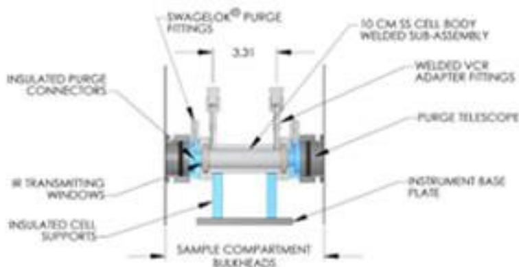
Short Path Gas cells are useful for pure gases and, generally speaking, for concentrations of not less than 100 ppm. Cell utility for various ppm concentrations is dependent not only on path length, but also on the absorbance characteristics of the sample. Feel free to consult with us on these and any other issues concerning selection of an appropriate gas cell.
