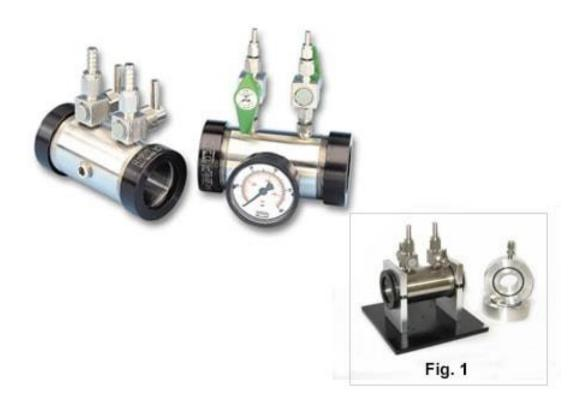
The G-2SS stainless steel gas cell is useful for qualitative analysis of pure gases and mixtures where one or more of the constituent gases are present in concentrations of at least 5 percent. It can be used in situations that make use of a glass cell impractical, such as applications involving high pressure or gases that etch a glass cell body.
