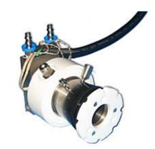
the cylinder permits the cell pathlength to be read within 0.0005mm (0.5 micrometer). In order for weaker absorption bands of many liquids to appear with the proper intensity, the stronger bands will be totally absorbed and their exact location thus obscured. In these situations, the Variable Pathlength Cell may be precisely adjusted to provide just the right intensity for exact location of both weak and strong bands.
