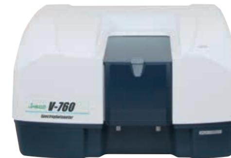
The V-760 double beam, double monochromator optical design with lowest stray light (0.00008 %) offers high absorbance linearity across the entire photometric range. The V-760 can measure up to 6 Abs in the UV-Visible region (and up to 8 Abs in the visible region\*). Variable spectral band width can be set down to 0.1 nm with special height slits to further reduce stray light and absorbance linearity is made even higher with rear beam attenuation.
