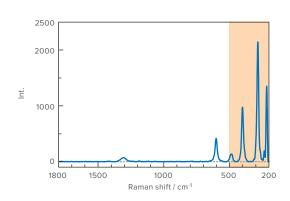
PR-1w allows to perform the low wavenumber measurement down to 200 cm<sup>-1</sup>.
