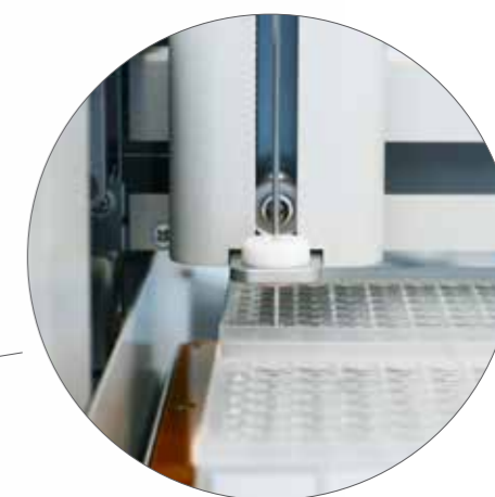
Sampling Nozzle with bias for piercing the plate sealer without risk of including debris.
