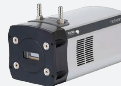
Detector Option: EMCCD Exposure as fast as 1 ms
