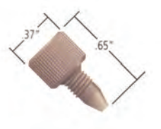
UP-F-127 10-32 PEEK™ Fitting Max Pressure 414 bar
